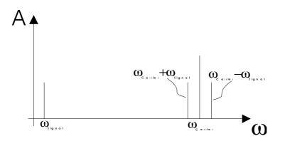
figure 2 - Standard Amplitude modulation
