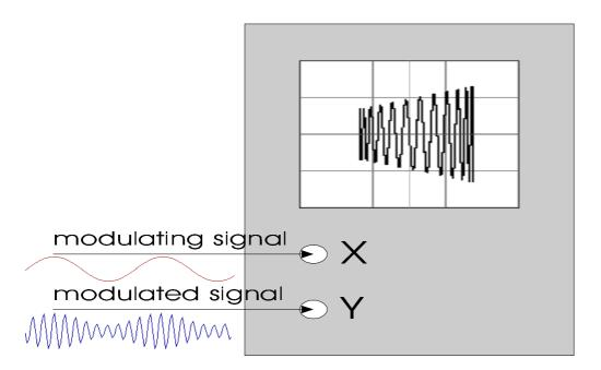
where m is called the modulation index (ratio of peak modulating signal to peak carrier signal), and A is the amplitude of the carrier signal.
