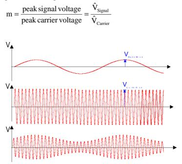
The above figure shows the connection between the modulating signal, the carrier signal and the modulation index m and how to measure via a usual oscilloscope.
