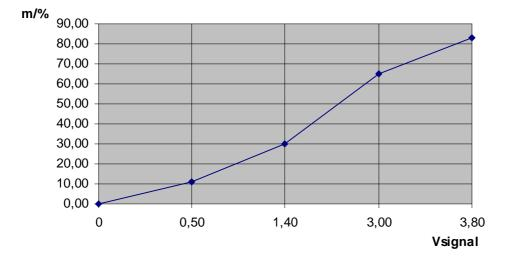
The above graph shows the modulation depth versus the signal amplitude obtained from the trapezium display.
