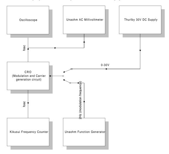
The CRO unit generates the carries frequency and contains a built in varicap diode and a calibrated capacitor with which the carrier frequency can be either manually or electronically be changed by applying a voltage to the varicap. A Thurlby 30V DC power supply and a Unaohm frequency generator can generate an appropriate voltage therefore.
