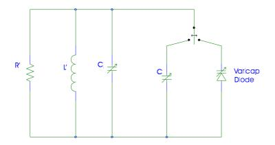
The left part of the circuit has got a fixed resonant frequency  $f_0$ . By applying the right part of the circuit it is possible to change this frequency  $f_0$  by either changing the value of C or the varicap diode by applying a suitable voltage to it.
