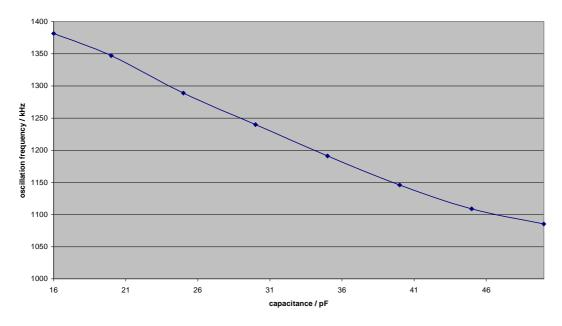
The variance of the capacitance C results in a nearly linear variance of the resonance frequency.
