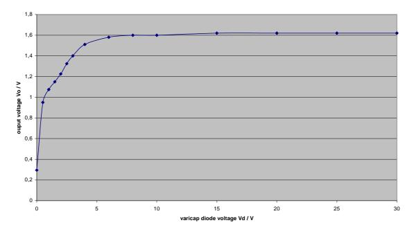
The output voltage is not at a stable level when only small voltages (low frequencies) are applied to the varicap. This results from the inner structure of the CRO.
