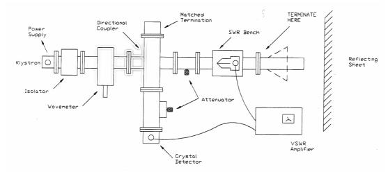
The lab equipment consists of a Klystron, as a microwave source, a directional coupler, an SWR Bench, a VSWR meter. Different terminations can be applied to the equipment, which were a matched termination, a short circuit and an open circuit and a matched horn aerial with reflector to measure the wavelength.
