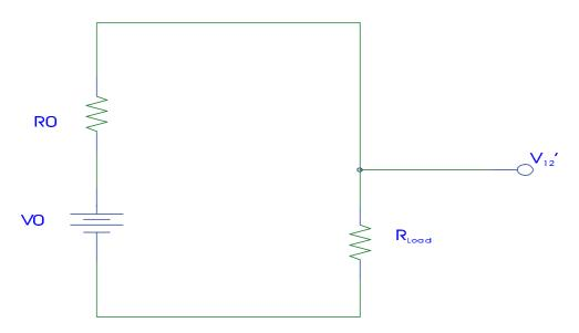
The output voltages of the bridge change when the bridge is connected to the opamp stage because the amplifier inputs are a load to the bridge. The new bridge output voltages can be calculated using Thevenin's theorem, where  $V_0$  is the disconnected bridge voltage.
