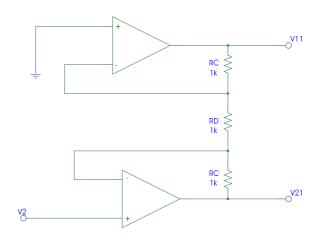
$$\frac{V_{21}}{V_2} = \frac{R_C + R_D}{R_D}$$
