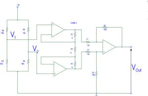
The output voltages of the bridge decrease when connecting to the opamp-circuit because of it's load function. The measured output values of the connected bridge were:  $V_1$ '=5.35V  $V_2$ '=5.32V at an output voltage  $V_{Out}$ =513mV
