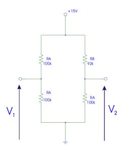
The bridge outputs were  $V_1=7.5V$  and  $V_2=7.67V$ . The calculated bridge voltages are:
