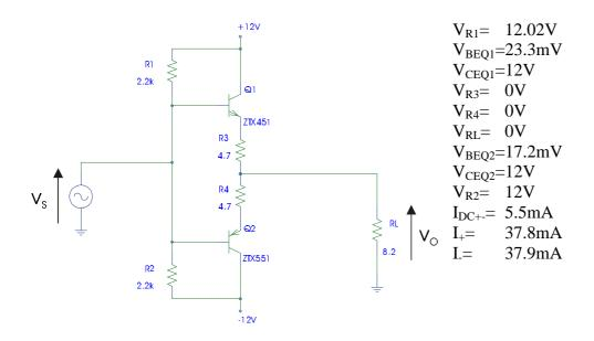
The DC-Bias shows, that there is no current through the transistors without a signal voltage  $v_s$  because the base inputs are short circuited. The current of about 5.5mA is caused only through the base resistors  $R_1$  and  $R_2$ . <u>I</u>=(V<sub>CC1</sub>+V<sub>CC2</sub>)/( $R_1$ + $R_2$ )=<u>5.45mA</u>.
