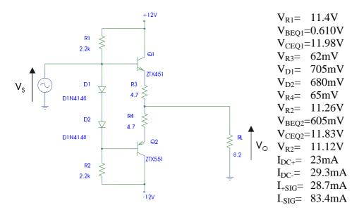
Now the current throug the different resistors can be determined:
