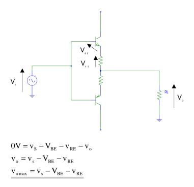
So the signal voltage, which is put to the enput of the push-pull amplifier has to be properly amplified (~ to the region of  $V_{CC}$ ) for getting the maximum power output. This is valid for ALL "common collector" push-pull amplifiers and is only once shown here.
