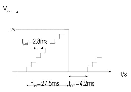
The measured values are close to the calculated. some differences come from the non ideal resistors and capacitors, which had not all their desired values (+- 5per cent).
