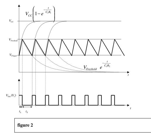
Figure 2 shows how the Astable with the Timer NE55 works. The  $0.1\mu$ F capacitor is charged through R<sub>1</sub> and discharged through R<sub>2</sub> and Pin 7 (Discharge Input of NE555). The two diodes prevent the resistors from influence of each other (Exact duty times). When the voltage at the capacitor increases the threshold voltage of the NE555 (2/3 V<sub>CC</sub>), the output switched to 0V until the capacitor voltage decreases the trigger voltage at Pin 2 (1/3 V<sub>CC</sub>).
