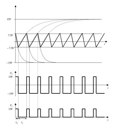
The Astable B works in a similar way than the other one. The  $0.1\mu$ F capacitor is charged through  $R_A$  and discharged through  $R_B$ . When increasing or decreasing the positive or negative voltage at the + input of the LM741, the 741 switches to the opposite state (Comparator mode). The diode at the output suppresses the negative parts of the output voltage.
