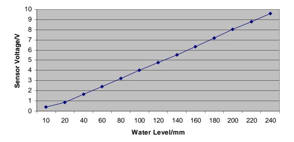
The liquid level sensors works linear – A higher liquid level provides a proportional higher output voltage.
