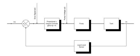
The combination of the integral and the proportional controller brings an improvement to the system by reducing the final error e. Now the output reaches the desired input (6V==150mm). The integral part brings a short oscillation with over and- under-shots to the system before it settles.
