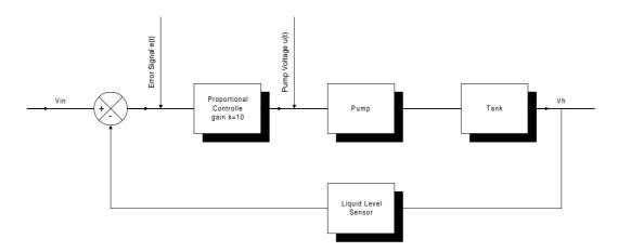
With the proportional control only the difference of the actual liquid-level and the input voltage (error signal) is amplified and directly fed to the pump. Therefore the proportional control doesn't reach the desired setting point of 150mm, because the end value depends very much on the value of k. The following plot from the oscilloscope shows this.
