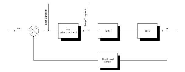
From the other parts it should be expected, that a combination of all three controllers brings the best result, but the transient response shows, that the settling time t increases and the systems tends to oscillate.
