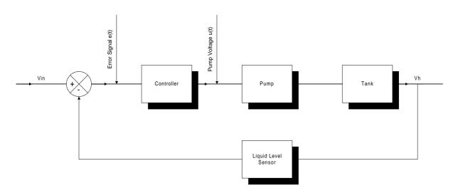
The schematic above shows the block diagram of the used liquid level control system. The controller drives the pump which fills the tank with water. The backward signal transfers the water level back to the input. The controller could be changed in its characteristics between proportional. integral. derivative. some of them and all together to change the properties of the control-process.
