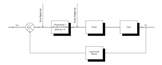
Adding a derivative controller to the proportional one brings no big difference. The output never reaches the desired input value and the derivative controller brings no improvement to the time constant or the settling time.
