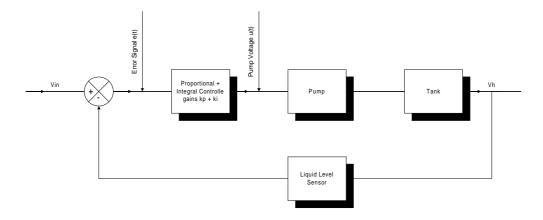
The overall performance of the system increases, when the integral part is reduced and the proportional factor is left constant. This reduces the oscillating and results only in one overshot, after which the outputs settles to its desired value.
