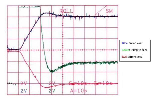
At the beginning the pump voltage increases to its maximum. Then, when the output reaches its desired value the pump-voltage drops, the output overshoots and due to the negative error signal the output decreases until it has settled down to the end-value of 150mm or 6V. So the PI controller is the best solution for this system.
