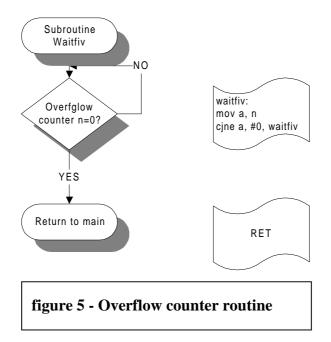
The overflow counter routine is called at the end of the main program in order to secure a proper timing.
