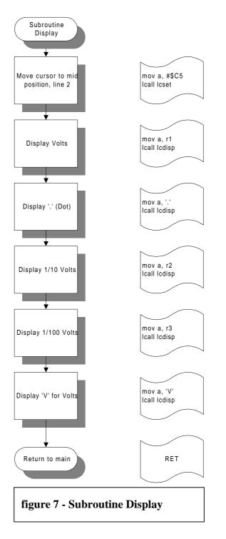
Figure 7 shows the subroutine to display the stored data on the LC-Display. First the cursor is moved to a mid position in the second row via the LCSET function, and then the registers are output in the format #.##V, like on a usual DVM.
