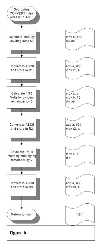
Figure 6 shows the flowchart of the scaling procedure. The different digits are stored in the registers R1..R3.
