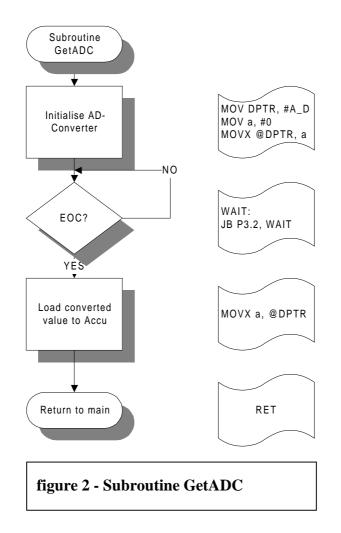
Figure 2 shows the flowchart for the subroutine, which reads from the ADC and writes it to the Accumulator.
